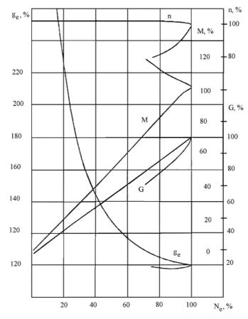
Fig. 1. Generalised load curves of the tractor diesel engines:  $N_e$  – efficient power, %; n – rotational speed of the crankshaft, %; M – moment of rotation, %;  $g_e$  – specific fuel consumption related to a unit of work of engine, %; G – total fuel consumption per unit of time, %
