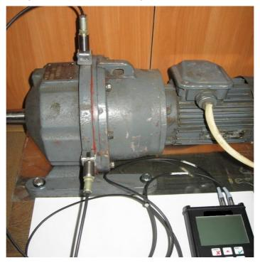
Fig. 1. Planetary reduction gearmotor
