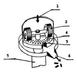
a) 1 – material feed, 2 – rotating extrusion cylinders,
