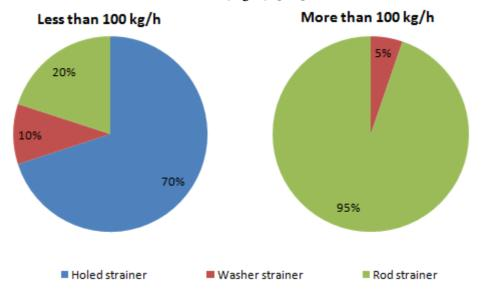
Fig. 7. The percentage of oil-pressing equipment according to strainer constructions
