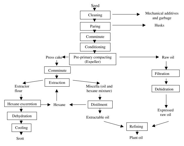
Fig. 1. Processing oil-seed in (central) industrial oil hall
