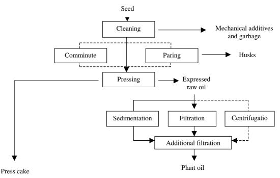
Fig. 2. Processing oil-seed in (local) small devices
