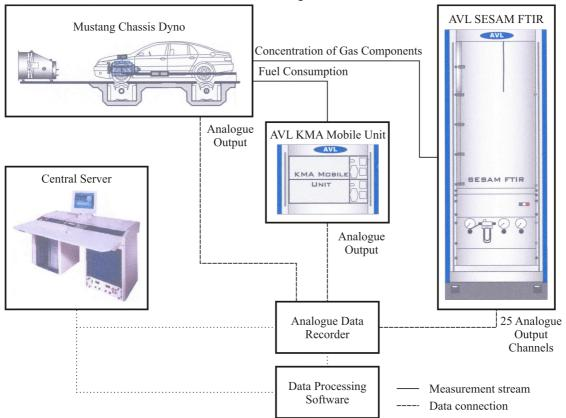
Fig. 4. Block diagram for the diagnostic test and emission test routines
