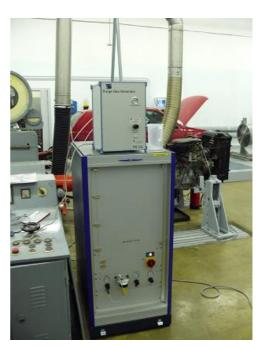
Fig. 5. AVL SESAM FTIR Exhaust Gas Measurement System
