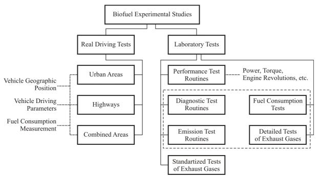
Fig. 1. Flow chart of the procedure for automobile testing
