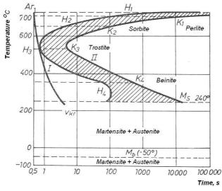
Fig. 6. Curve of austenite isothermal transformation
