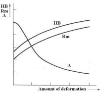
Fig. 3. Influence of deformations on mechanical properties of materials
