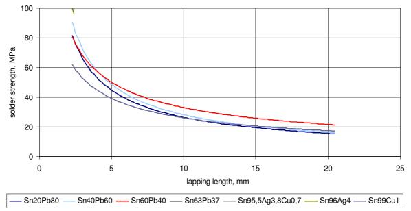
Fig. 3. Relation between the solder strength and lapping length
