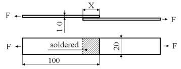
Fig. 1. Dimensions of the test assembly
