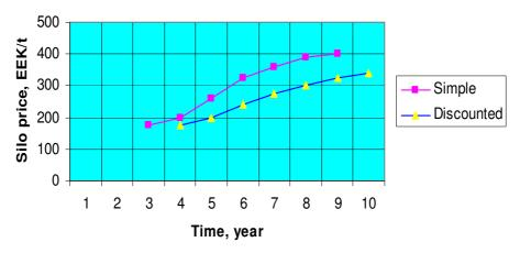
Fig. 1. Simple and discounted payback time depending on the silo price (electric sales tariff 1.25 EEK kWh<sup>-1</sup>)
