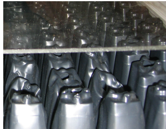
Fig. 2. Sun heated collector with 12 seed box absorber
