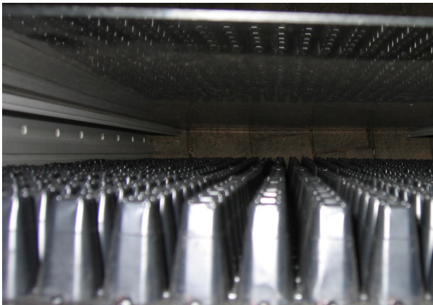
Fig. 1. Sun heated collector with 22 seed box absorber
