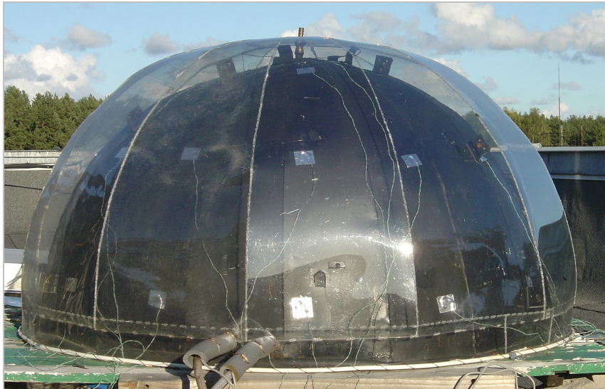
Fig. 1. Semi-spherical solar collector
