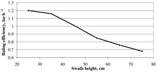
Fig.3. Baling efficiency depending on the height of the shaft
