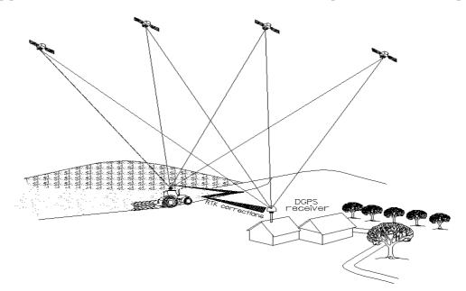
Fig. 1. Precise DGPS data acquisition individual system
