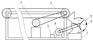
Fig.1. Schematic overview of the structural parameters and performance indicators of the vanetype rethresher experimental unit: 1, 4 – electric motors; 2 – belt-conveyor; 3 – power meter; 5 – rotor of the rethresher; 6 – toothed concave; 7 – tailings collection container
