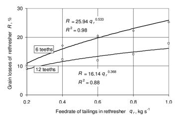
Fig. 7. Influence of tailings feed rate in the rethresher  $q_r$  to the grain losses of the rethresher R
