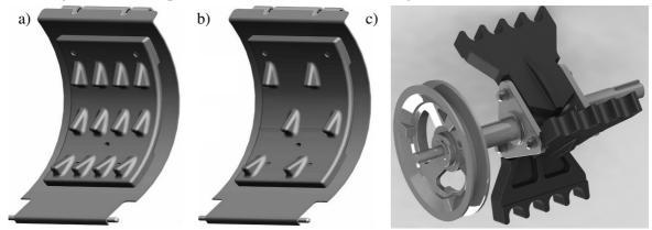
Fig. 2. Concaves of the ear rethresher (a) and (b) and the rotor (c)
