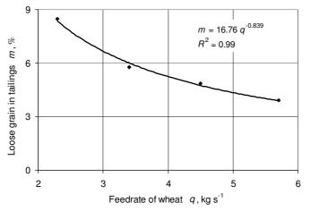
Fig. 3. Influence of wheat feed rate of the combine harvester *q* to the loose grain part in the rethresher *m*
