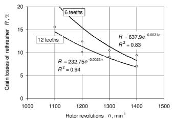
Fig. 4. Influence of rethresher rotor revolutions *n* to the grain losses of the rethresher *R*
