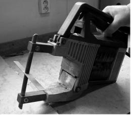
Fig. 1. Regulator of resistance electrode holder – soft mode
