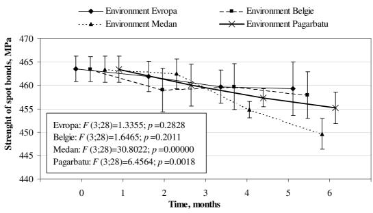
Fig. 6. Influence of time and environment on strength of spot bonds
