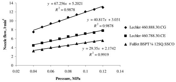
Fig. 2. Measurement of water nozzle flow
