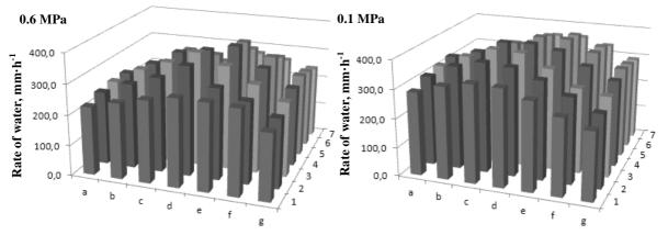
Fig. 4. Progression of surface unevenness of the nozzle Lechler 460.888.30.CG
