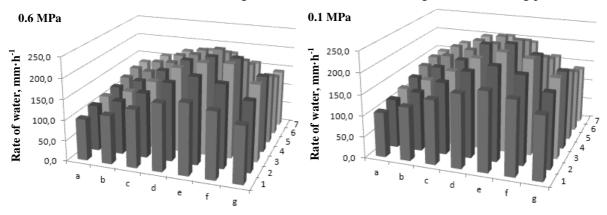
Fig. 3. Progression of surface unevenness of the nozzle Lechler 460.788.30.CE
