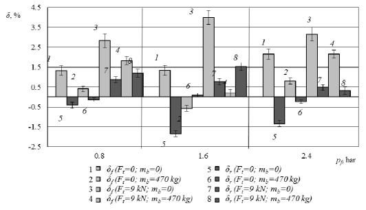
Fig. 1. Dependence of slippage of the front  $\delta_f$  and rear  $\delta_r$  wheels of the tractor on different air pressure in the front tires  $p_f$  driving without ballast ( $m_b = 0$ ), with ballast ( $m_b = 470$  kg), without tractive force ( $F_t = 0$ ), loaded with tractive force ( $F_t = 9$  kN); Inflation pressure in the front tires  $p_f$ : 0.8; 1.6; 2.4 bar
