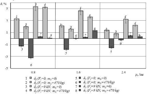
Fig. 2. Dependence of slippage of the front  $\delta_f$  and rear  $\delta_r$  wheels of the tractor on different inflation pressure in the rear tires  $p_r$  driving without ballast ( $m_b = 0$ ), with ballast ( $m_b = 470$  kg), without tractive force ( $F_t = 0$ ), loaded with tractive force ( $F_t = 9$  kN); inflation pressure in the rear tires  $p_r$ : 0.8; 1.6; 2.4 bar
