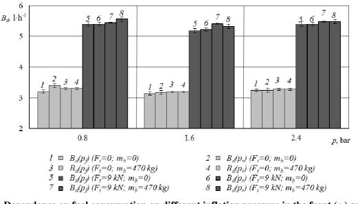
Fig. 4. Dependence on fuel consumption on different inflation pressure in the front  $(p_f)$  and rear  $(p_r)$  tires driving without ballast  $(m_b = 0)$ , with ballast  $(m_b = 470 \text{ kg})$ , without tractive force  $(F_t = 0)$ , loaded with tractive force  $(F_t = 9 \text{ kN})$ ; the inflation pressure in the tires p: 0.8; 1.6; 2.4 bar
