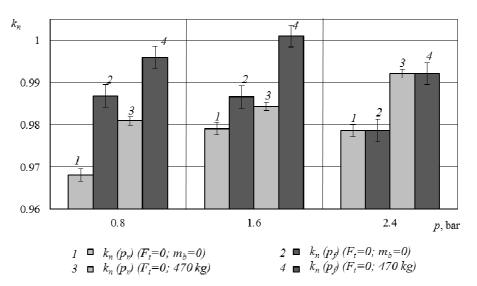
Fig. 3. Kinematic discrepancy  $k_n$  of the driving wheels of the tractor driving without ballast  $(m_b = 0)$ , with ballast  $(m_b = 470 \text{ kg})$  on different inflation pressure on the front  $(p_f)$  and rear  $(p_r)$  driving wheels: 0.8; 1.6; 2.4 bar
