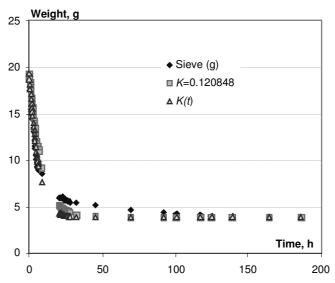
Fig. 6. Sambucus nigra L. flower weight change (experimental and theoretical calculated) during drying on a sieve
