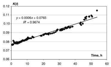
Fig. 3. Linden (Tilia cordata L.) flowers' drying rate determination, drying it on a sieve
