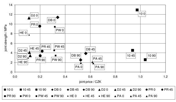
Fig. 3. Strength and price of bonded joints at the use of different adhesives
