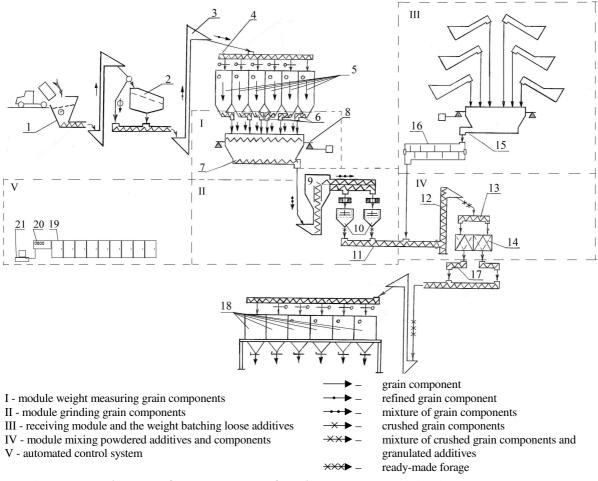
Fig. 1. **Flow diagram of a modular set of equipment:** 1 – receiving hopper; 2 – separator; 3 – elevator; 4, 13 – infeed conveyor; 5, 18 – bunker; 6, 17 – unloading conveyors; 7, 15 – weight bin; 8 – load cells; 9–bin active; 10 – crusher; 11 – modular conveyor; 12 – vertical conveyor; 14, 16 – mixer; 19 – electrical cabinet; 20 – control cabinet; 21 – remote control
