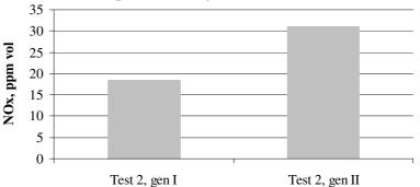
Fig. 9. Comparison of the amounts of NOx contained in exhaust gases in Test 2
