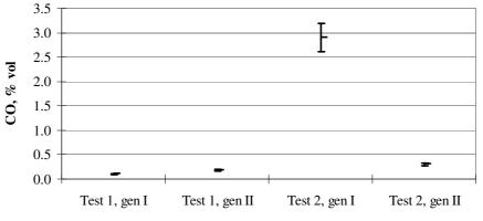
Fig. 6. Comparison of the amounts of CO contained in exhaust gases
