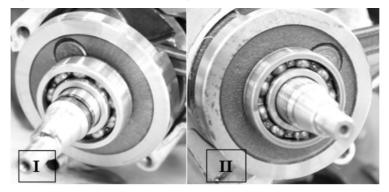
Fig. 5. Comparison of corrosion with the tested generators I and II
