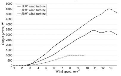
Fig. 3. Power curves for 3 type wind turbines with rated power 1 kW, 3 kW, 5 kW [6]
