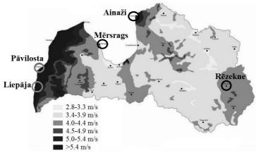
Fig. 4. Average yearly wind speed in Latvia 10 meter height [7]
