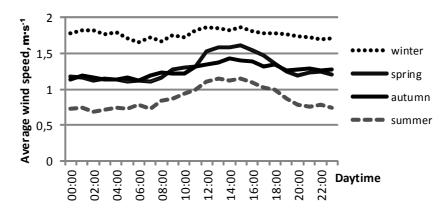
Fig. 2. Average hourly wind speed in Liepaja (Latvia) 10 meter height [5]
