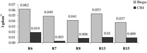
Fig. 2. Biogas and methane l·g<sub>dom</sub><sup>-1</sup> add from digestate digested at 18 °C
