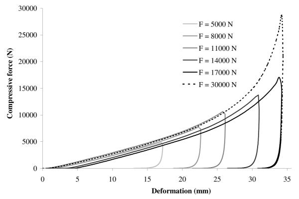
Fig. 2. Hysteresis curve for different values of maximal compressive force
