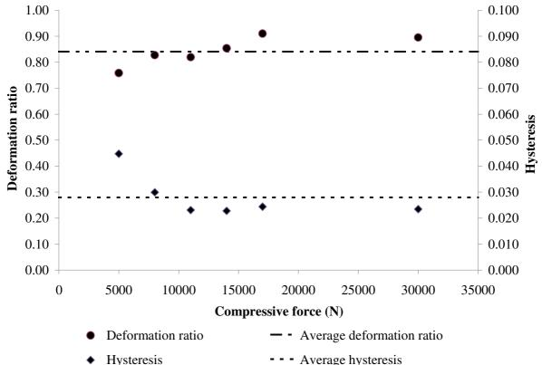
Fig. 3. Dependency of deformation ratio and hysteresis vesrsus compressive force
