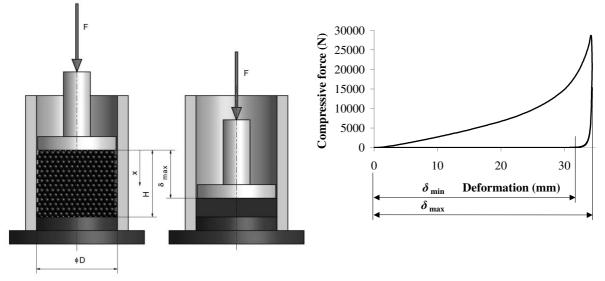
Fig. 1a. Scheme of pressing equipment
