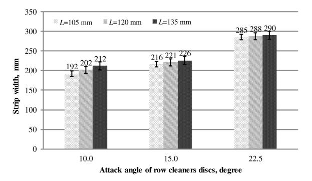
Fig. 2. Strip width dependence on technical parameters of the row cleaner
