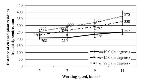
Fig. 3. Working speed and row cleaner attack angle influence on the cleaned off crop residues distance from the centre of the strip, where L = 105 mm
