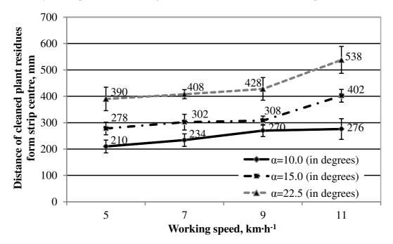
Fig. 4. Working speed and row cleaner attack angle influence on the cleaned off crop residues distance from the centre of the strip, where L = 120 mm
