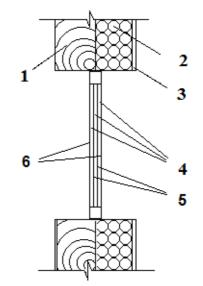
Fig. 1. Window opening with 2 windows: 1 – aero concrete wall; 2 – polystyrene insulation; 3 – wood finish; 4 – outside window; 5 – air space; 6 – inside window
