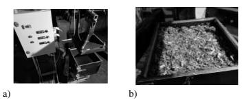
Fig. 5. Press for pressing the fleece material: a – pressing equipment; b – pressing chamber
