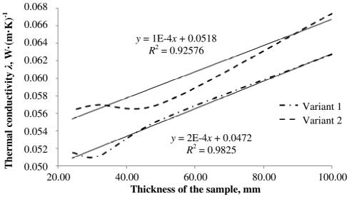
Fig. 8. Thermal conductivity of a slab depending on its thickness
