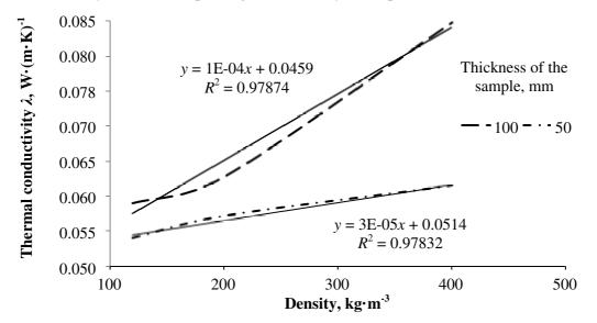
Fig. 7. Thermal conductivity of a slab depending on its density
