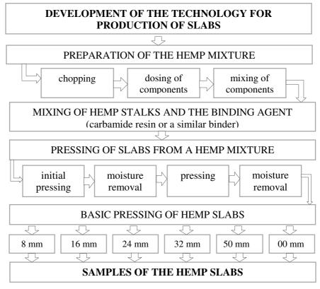
Fig.1. Scheme of the slab production technology
