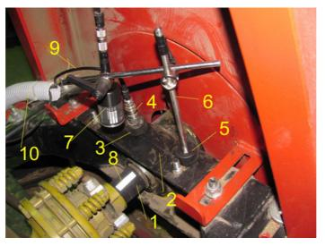
Fig. 2. Vibration sensor montage on bearing housing
