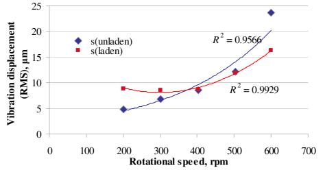
Fig. 6. Cutter head bearing housing vibration displacement (RMS) values
