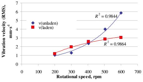
Fig. 5. Cutter head bearing housing vibration velocity (RMS) values
