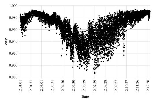
Fig. 3. Power factor  $\cos\varphi = f(t)$  calculated from collected data
