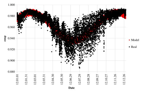
Fig. 4. Mathematic model  $\cos\varphi = f(t)$  application on observed power factor data
