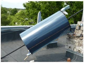
Fig. 1. Cylindrical solar collector
