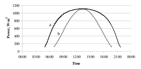
Fig. 5. Theoretically calculated daily course of power of solar collectors: a – cylindrical; b – flat
