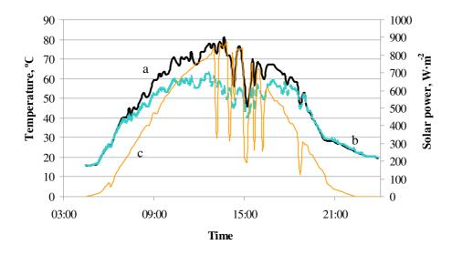
Fig. 6. Daily course of temperature of air outflowing from cylindrical solar collector (a and b) and global solar power (c)
