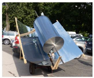
Fig. 2. Cylindrical solar collector with reflector
