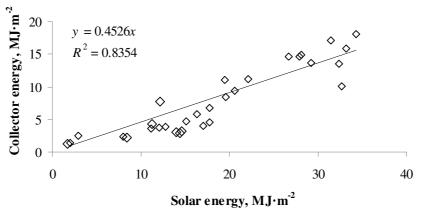
Fig. 8. Dependence of daily sum of energy output from cylindrical solar collector on daily sum of global solar energy
