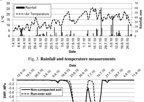
Fig. 4. Soil water potential from depth of 100-122 mm
