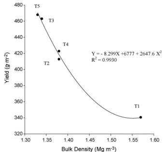
Fig. 1. Relationship between soil bulk density and grain yield of wheat [12]
