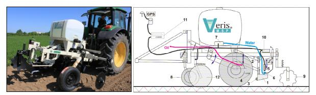
Fig. 1. Veris MSP machine with Soil pH Manager system: 1 – scoop; 2 – mechanism of scoop lifting; 3 – adapter; 4 – hog; 5 – pH sensors; 6 – water supply with nozzles; 7 – water tank; 8 – plant residues removal; 9 – furrow filling hoes; 10 – controller; 11 – data recorder; 12 – sensor of soil electrical conductivity
