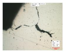
Fig. 12. Oxide membranes, inclusions
