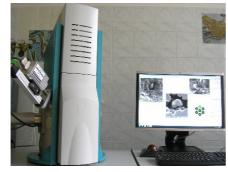
Fig.7. Electron microscope Tescan Vega 3
