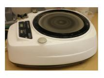
Fig. 5. Grinding and polishing machine MTH Kompakt 1031
