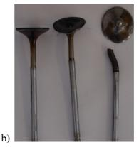
Fig. 9. Examples of the analysed components: a – part of the car chassis, fracture; b – valves, creep
