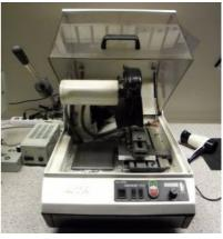
Fig. 3. Metallographic saw MTH Mikron 110
