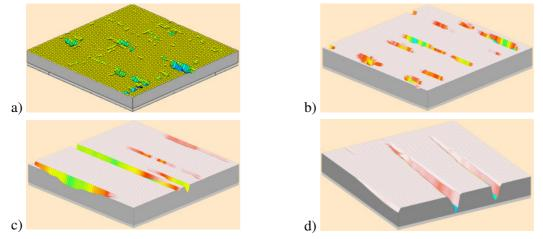
Fig. 7. Roughness of surfaces No.1 (a), No.3 (b), No.6 (c), No.8 (d) after the stage of normal wear
