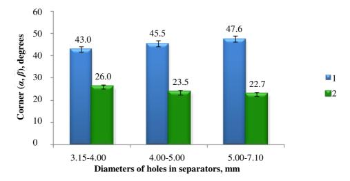
Fig. 3. Natural slope and inrush failure angle dependency on granule diameter: 1 – natural slope angle ( $\alpha$ ); 2 – inrush failure angle ( $\beta$ )
