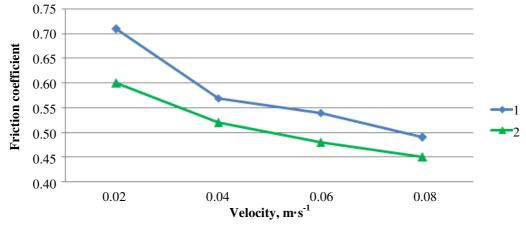
Fig. 1. Granule kinetic friction coefficient dependency on sliding velocity on metal surface: 1-4 mm diameter granules; 2-6 mm diameter granules
