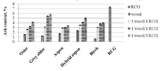
Fig. 3. Ash content in reed canary grass and timber pellets
