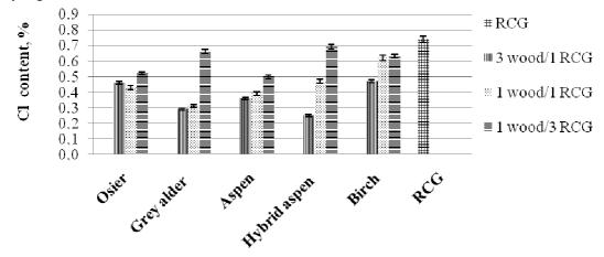
Fig. 2. Chlorine content in reed canary grass and timber pellets
