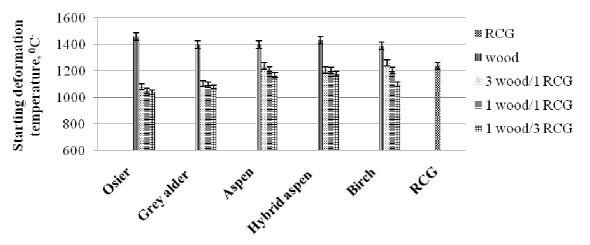
Fig. 4. Starting deformation temperature of reed canary grass and timber pellets
