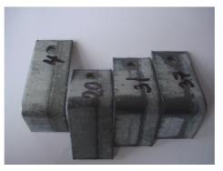
Fig. 6. Corrosion signs on the samples (sample No.4 was exposed to the acid for 24 h, No.20 – for 48 h, No.31 – for 72 h and No.37 – for 96 h)
