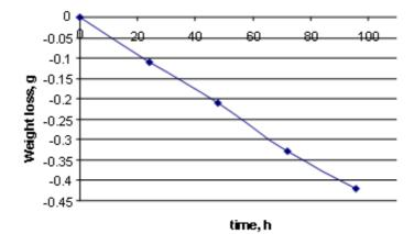
Fig. 5. Weight losses of the zinc galvanised samples exposed to a 5 % acetic acid anhydride solution
