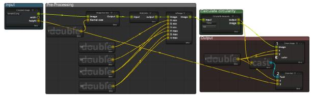
Fig. 6. Computer vision system as seen in the framework for finding circularity of tomatoes
