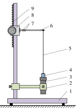
Fig. 3. Scheme of the experimental facility: 1 – stanchion; 2 – binding; 3 – plunger liner; 4 – plunger; 5 – flexible string; 6 – power sensor; 7 – resistance strain gauges; 8 – hand wheel; 9 – rack
