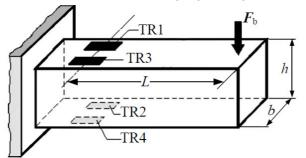
Fig. 4. Force sensor structure: TR1, TR2, TR3, TR4 – resistance strain gauges; L –distance between the center of attachment of resistance strain gauge to the location where the force is applied;  $F_b$  – applied force; h – height of the metal plate; b – width of the metal plate
