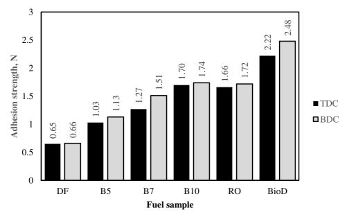
Fig. 6. Agglutination force measurement results
