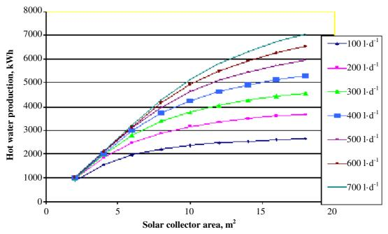
Fig. 4. Diagrams of hot water production depending on solar collectors area
