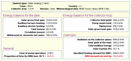
Fig. 3. Total energy balance for boiler and solar collectors
