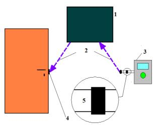
Fig. 1. Sabotage of the system with central logic: 1 – central unit; 2 – inaccessible wiring; 3 – reader; 4 – electrical lock; 5 – module for scanning the bus
