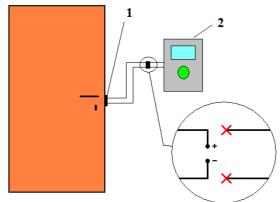
Fig. 2. Sabotage of the system with direct control: 1 - electrical lock; 2 - reader
