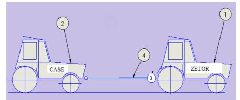
Fig. 1. **Research scheme:** 1 – tractor Case IH Farmall U Pro 115; 2 – tractor Zetor 10540; 3 – pulling force measurement device; 4 – rigid connection
