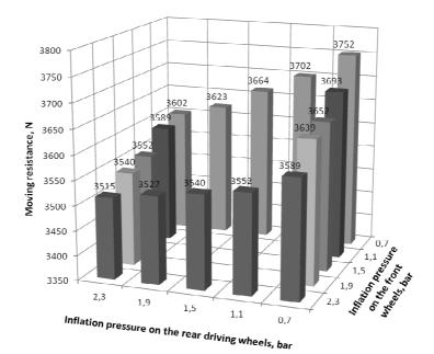
Fig. 3. Tractor 4x2 moving resistance force dependences on different inflation pressure on the front and rear tires on hard surface road
