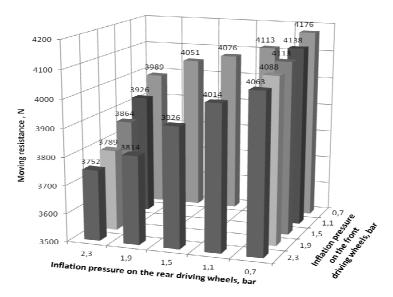
Fig. 4. Tractor 4x4 moving resistance force dependences on different inflation pressure on the front and rear tires on hard surface road
