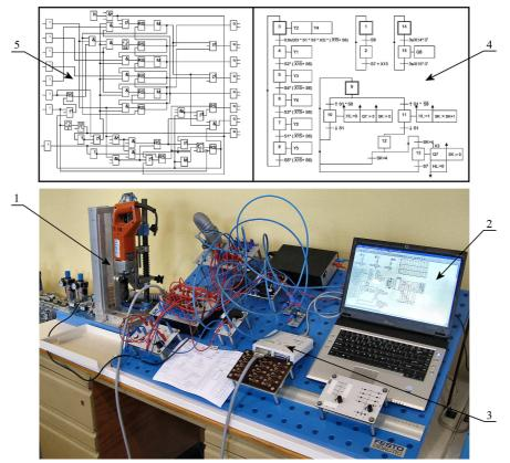
Fig. 1. Festo Didactic learning stand with automatic drilling machine: 1 – drill with preforms magazine; 2 – a computer with FluidSIM software; 3 – EasyPort; 4 – the control algorithm and program Grafcet form; 5 – the control program in the form of FBD
