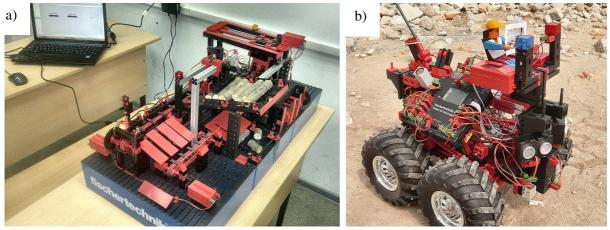
Fig. 2. Mockups from Fischertechnik constructors equipment elements: a – automated timber sorting machine; b – autonomous robot/tractor model with GPS Navigation
