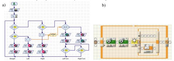
Fig. 3. **Designed graphical programming languages for beginners:** a – Fischertechnik Robot Pro programming language; b – Lego Mindstorms graphic programming language
