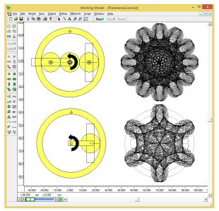
Fig. 4. Planetary mechanism of computer simulation with Working Model
