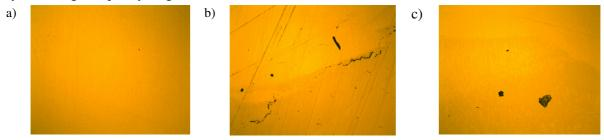
Fig. 7. MMA welded layers (x100): a – good fusion; b – non-fusion; c – inclusions
