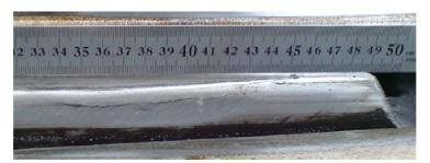
Fig. 3. Longitudial cracks on frog point after second build-up welding
