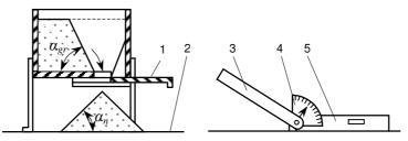
Fig. 1. Scheme of determination equipment of natural slope and fall angles: 1 – damper; 2 – horizontal surface; 3 – turning ruler; 4 – protractor; 5 – ruler with level
