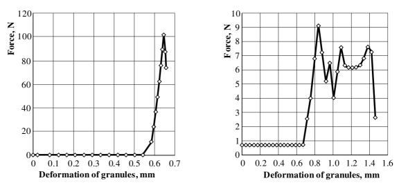
Fig. 3. Deformation (mm) and disintegration force (N) of granulated Kieserite granules
