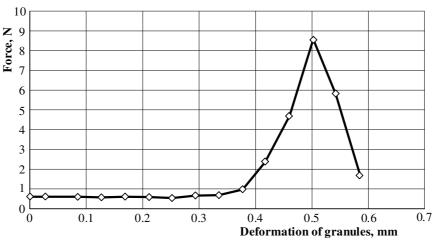
Fig. 5. Deformation (mm) and disintegration force (N) of granulated Serpentine smaller-size granules
