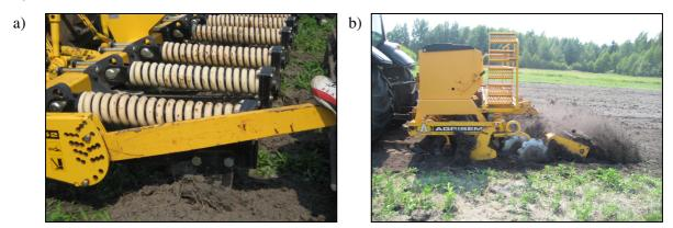
Fig 1. **Tillage and sowing equipment:** a – subsoiler Agrisem Combiplow; b – drill for scattered sowing Agrisem Disc-O-Sem
