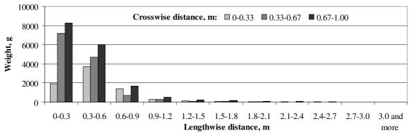
Fig. 4. Particle translocation in the particular segments for conventional technology
