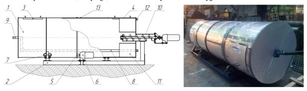
Fig. 3. Breadboard model of an experimental biofermentation installation of the drum type:
