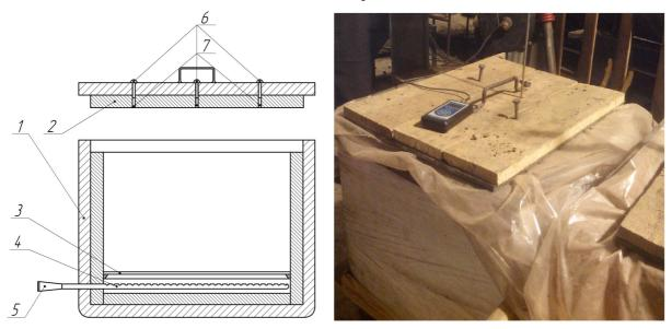
Fig. 2. Breadboard model of an experimental biofermentation installation of the chamber type: 1 – biofermentor chamber; 2 – removable lid; 3 – perforated plate; 4 – perforated zigzag pipe; 5 – air compressor nozzle; 6 – plugs; 7 – holes for temperature and oxygen content measurements
