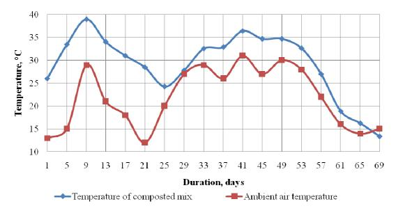
Fig. 4. Graph of the temperature dynamics pattern under the passive pile composting
