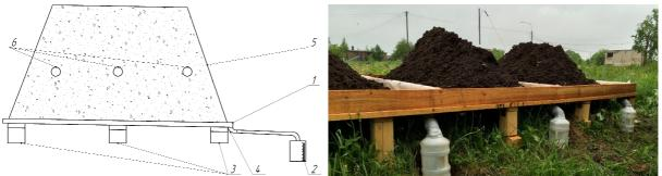
Fig. 1. Experimental ground for field-edge composting: 1 – base; 2 – vessel to accumulate and measure effluents; 3 – support; 4 – moisture trap; 5 – compost mix; 6 – sampling and temperature measurement points
