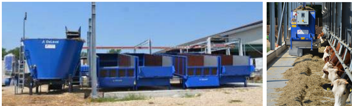
Fig. 2. Components of the AFS: the TMR mixing unit, the feeding hoppers (left) and the distribution wagon (right)
