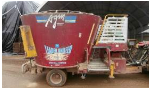
Fig. 1. Conventional feeding system (CFS) represented by a trailed mixer wagon, equipped with a single, vertical axis auger
