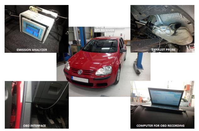
Fig. 1. Equipment of measuring vehicle
