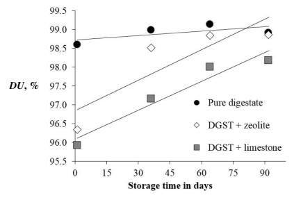
Fig. 2. Process of mechanical durability change during storage time
