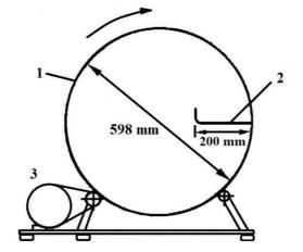
Fig. 1. Rotary drum: 1 – drum; 2 – partition; 3 – motor
